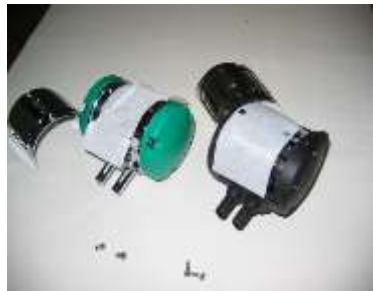
How to replace the lid of the pulsator
